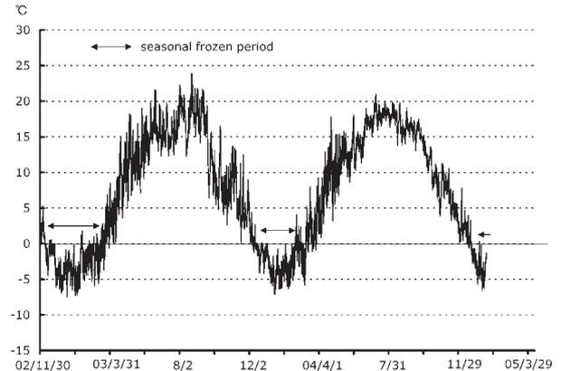
Fig. 6 Rock surface temperature at Point 1
