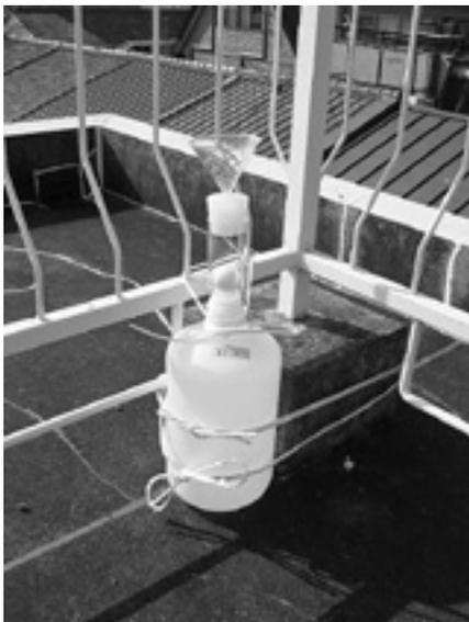
Photo 1 Precipitation sampler installed on P-1
