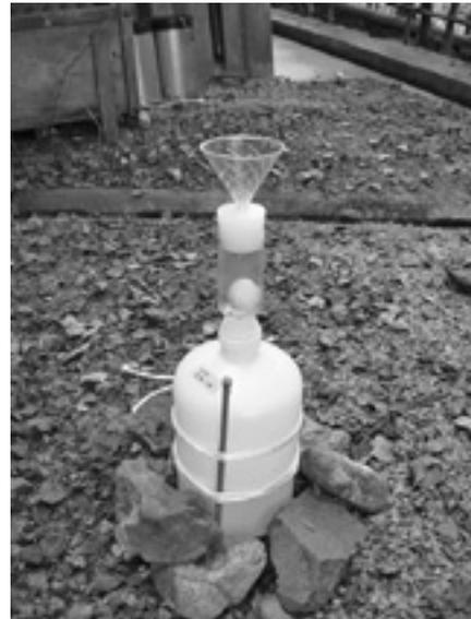
Photo 3 Precipitation sampler installed on P-3
