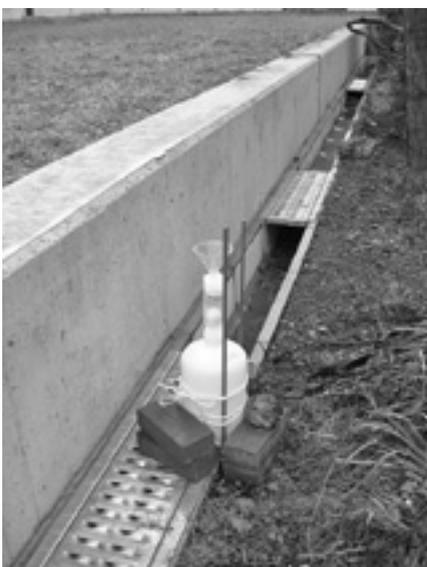
Photo 2 Precipitation sampler installed on P-2
